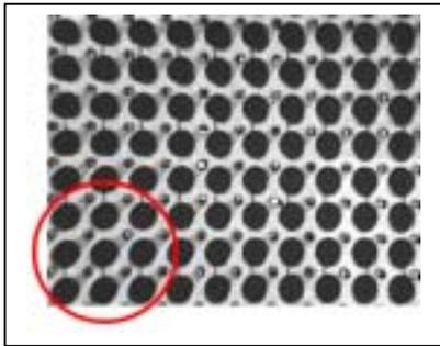
**5A and 5B** Elliptical X-ray images, the signature of insufficient reflow.
