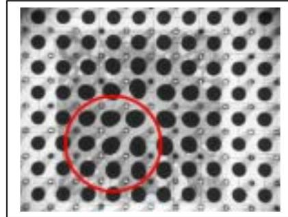
**Figure 7A** Doming (7A) and dishing (7B), the signatures of BGA package deformation, with (7C) showing a visual microscope image of a ball breaking away from the package.
