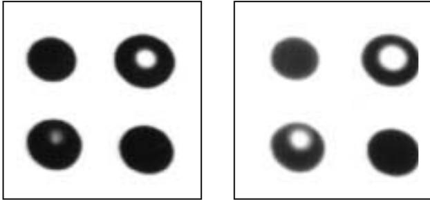
**Figure 8** The Voltage Blooming effect, showing the same void appearing to be larger at 60kV than at 50kV.
