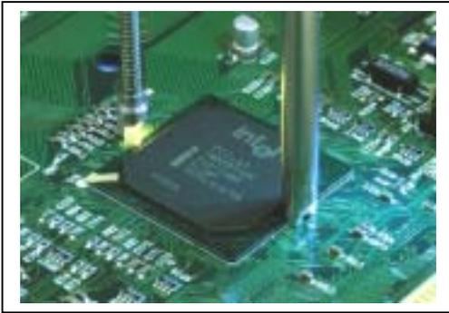
**Figure 10A** An endoscopic inspection system (10A) and its resulting image (10B).
