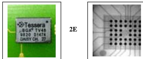
**Figure 2** Examples of BGA package types: Plastic BGA (2A), Super BGA (2B), Ceramic BGA (2C), Tab BGA (2D) and Micro BGA (2E).
