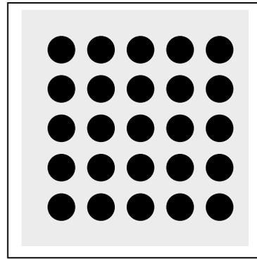
**Figure 4** BGA uniformity, the ideal reflow result.
