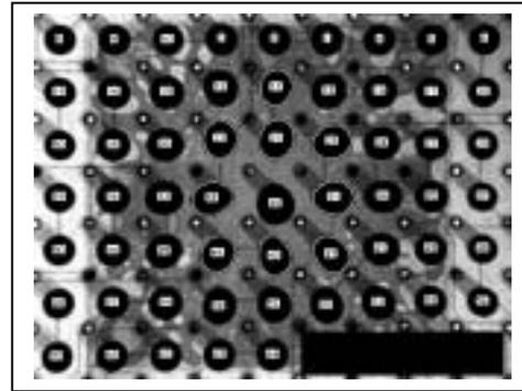
**Figure 9** Image processing software can highlight and flag deviant signatures rapidly and repeatedly.
