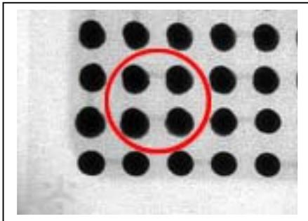
**Figure 6** Irregular X-ray images, the signature of cold solder joints.
