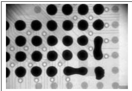
**Figure 1A** Examples of typical defects in BGA assembly: bridging, missing balls and solder voids: “Bridging”
